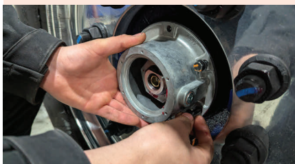
Step 5. Install metal hub cap to the hub (as supplied in kit). 6. Fill metal hub cap with SEMI
