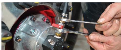
IMPORTANT NOTE Use 2 spanners on nuts and tails.
