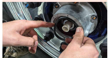
Step 7. Install provided O ring into metal hub cap as shown.
