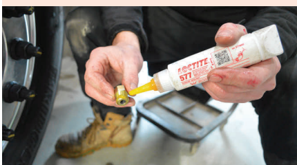
Step 3. Seal drive dog with LOCTITE 577. Install drive dog in stub axle.
