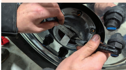
Step 4. Install white drive dog sleeve. Measure as shown in pic - Drive dog sleeve must be flush with metal cap. Cut to measured line, deburr the white sleeve. Install sleeve and double check length.
