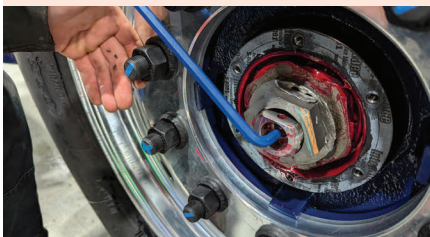
Step 2. Once removed, clean out grease and remove allen key plug in the stub axle.
