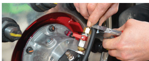
Tighten crimp clamp if hose leaks with side cutters.
