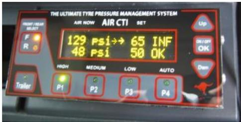
The unit is roughly 110mm x 45mm and allows the driver to select tyre-pressure modes to match terrain conditions. These modes are clearly seen in the attached photo as P1, P2, P3 while P4 is for an automated system. The unit displays current tyre pressures, selected modes and system status.
