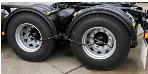
Fitted wheels have centre rotators which "rotate" with the tyre when the vehicle is in motion while allowing air pressure into the tyre.
